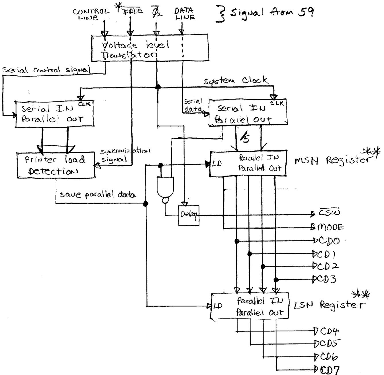
\* Note  $\overline{IDLE}$  is used as a serial data synchronization control signal
