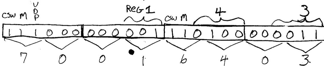
EXAMPLE 6 - Load VDP Register 1 with 67 then write 250, 103, and 25 to locations 3330, 3331 and 3332 respectively.
