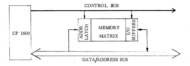
In system with larger memories, more sophisticated peripheral interfacing, and extensive modularity and expandability, the CP-1600 is best utilized with bipolar buffering of the bidirectional bus. Many standard, multiple-sourced, TTL parts are presently available for this purpose and provide the system designer with a number of important configuration options.
