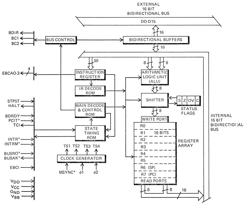
FIG. 2-2 INTERNAL BLOCK DIAGRAM
