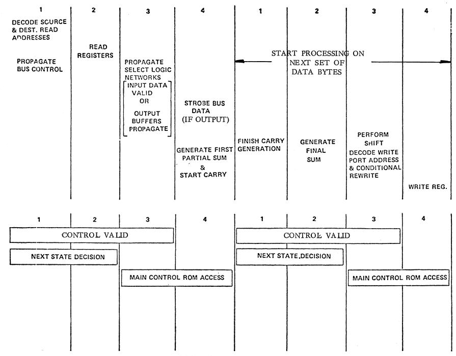
FIG. 2-4 PIPELINE TIMING
